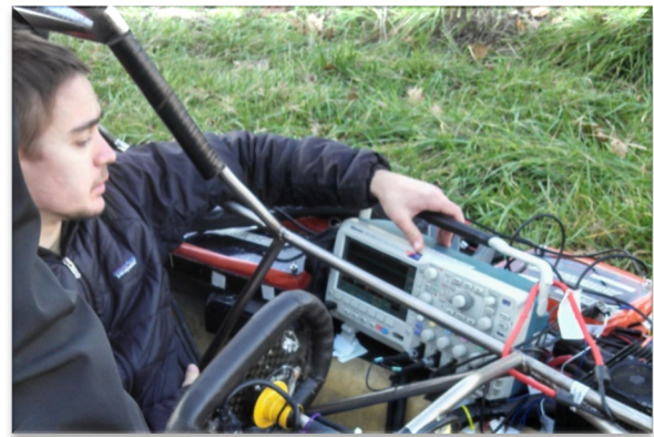
FIGURE 5: TESTING MOTOR BEHAVIOR UNDER NORMAL DRIVING CONDITIONS
