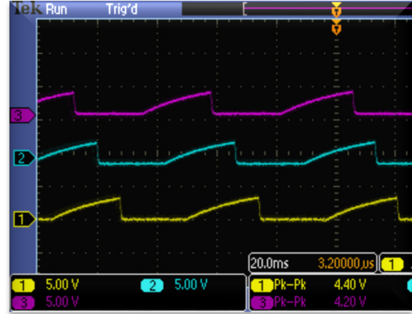
FIGURE 14: CHARGE DELAY DUE TO LOW PASS FILTER ON HALL EFFECT SIGNAL LINE
